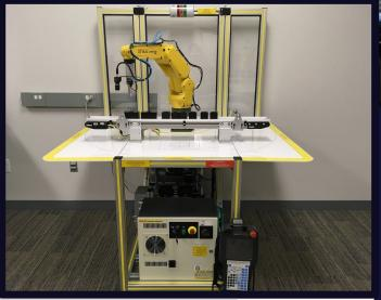
Our pre-engineered Robot Training Kits are designed to keep you Industry 4.0-ready. The surface fits most robot brands and multiple robot sizes. The mobile training design is ideal for classrooms, labs, and training centers and its versatility makes it the perfect solution for schools offering robotic, automation, or mechatronics programs.
